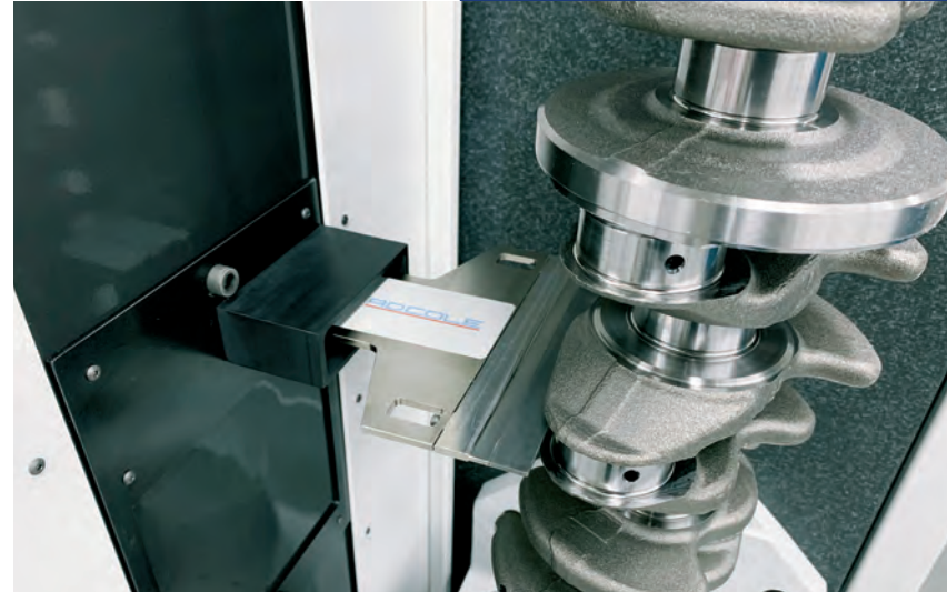
The 1100-S provides radial accuracies of \pm 0.5 \mu\text{m}
