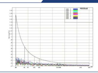
Sliding Window software enables users to capture the maximum amplitude portrayed across the entire chatter "burst" in the 120° window
