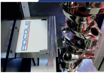
The **Adcole Model 1200-LX** is a high-speed, high-precision gage designed to measure camshafts, crankshafts, pistons, and other cylindrical components in demanding production environments. The heart of the 1200-LX is a laser interferometer, which enables the gage to measure to submicron accuracy and repeatability.
