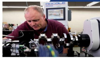
The Adcole Model 1000 is a high precision surface roughness measurement gage engineered to inspect camshafts, crankshafts and other precise cylindrical components. This horizontally loaded gage offers very fast surface measurement times, and delivers extremely accurate part measurement data.
