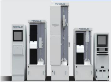
The DiaMetric<sup>TM</sup> follower system enables advanced manufacturers to obtain 5 times greater accuracy, achieving submicron performance levels of  $\pm$  .2  $\mu m$  when measuring diameters on their existing Adcole 911 gage<sup>i</sup>. Using the DiaMetric follower system, organizations can confidently measure concentric diameters on camshaft and crankshaft journals, eccentric shafts, robotic shafts and electric motor rotors with tolerances of <10  $\mu m$ .
